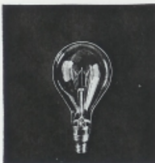
Movieflood, 2,000-watt P-S 52. Brings out blacks and blues. Primarily for color work. Used in regular 1,500-watt units. (15 hour life). About 1/10 size.
