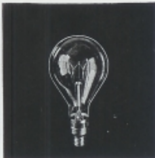
1,500 and 1,000-watt PS-52. Used in rifle lamps, side lamps and strip units. Also for floodlighting. About 1/10 size.
